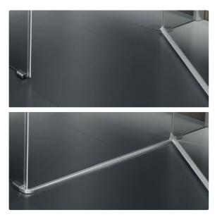
You can decide when installing the shower: 100% floor-level access or an optional 12 mm high surge bar, to give improved tightness in the door area.
