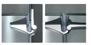
On opening inwards, the edge of the door pivots in the rounded cavity of the hinge and is then gently stopped by the sealant of the second glass part. When the door is closed, the two seals interlock, meaning that water leakage is effectively prevented.
